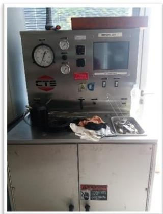
Gambar 2. Alat HPHT Consistometer CTE 22-400
