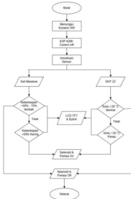
Gambar 3. Flowchart Alur kerja alat
